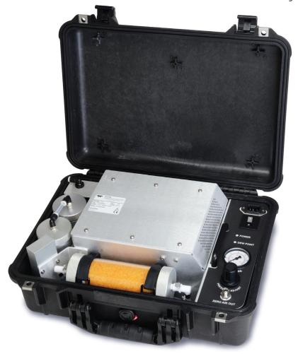
A fully self-contained portable source of clean, dry air for use with dilution calibrators, the Model 751 removes particulate and potential interferents from ambient air to create zero air suitable for calibration.
