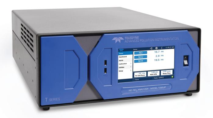
The Model T200UP provides Trace-Level measurements of NO,  $NO_x$  and  $NO_2$  using our Model T200U  $NO_x$  analyzer combined with a patented high efficiency Blue Light Converter (BLC). The BLC, also known as photolytic converter, provides a very specific conversion of  $NO_2$  with conversion efficiency similar to molybdenum.\*
