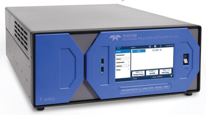
The Model T802  $O_2$  analyzer uses the proven paramagnetic measurement principle, coupled with state of the art microprocessor technology to provide accurate and dependable measurements of Percent Level  $O_2$ . The T802 offers a stable and inherently linear measurement of oxygen, making it possible to calibrate the analyzer by checking only two points. There is no requirement for a reference gas during operation.
