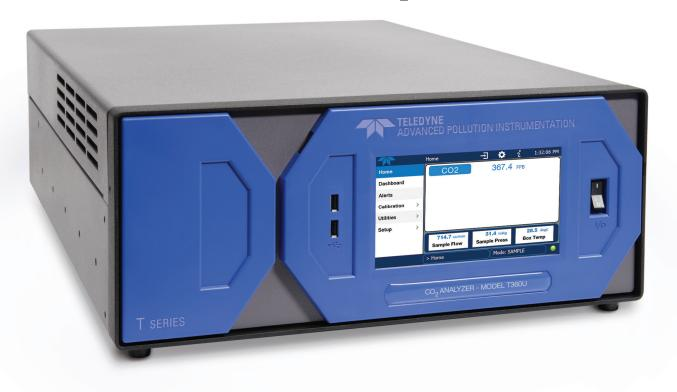
The Model 360U  $\mathrm{CO}_2$  analyzer measures of Carbon Dioxide by comparing infrared energy absorbed by a sample to that absorbed by a reference gas according to the Beer-Lamber law. Using a Gas Filter Correlation Wheel, a high energy IR light source is alternately passed through a  $\mathrm{CO}_2$  filled chamber and a chamber with no  $\mathrm{CO}_2$  present.
