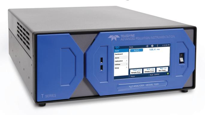
The Model T320  $N_2O$  analyzer measures Nitrous Oxide by comparing infrared energy absorbed by a sample to that absorbed by a reference gas according to the Beer-Lambert law. Using a Gas filter Correlation Wheel, a high energy IR light source is alternately passed through a  $N_2O$  filled chamber and a chamber with no  $N_2O$  present.
