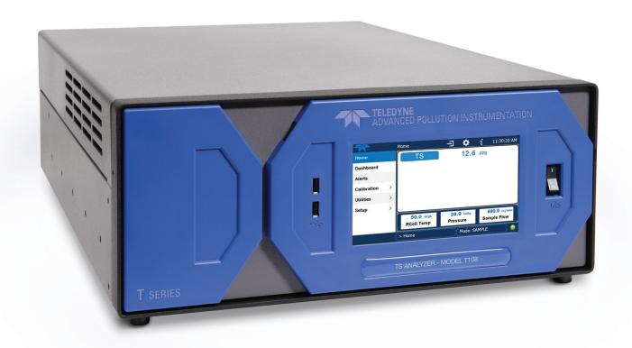
The Model T108 Total Sulfur analyzer is designed to measure mixed sulfur impurities, collectively referred to as Total Sulfides, in air or carbon dioxide gas. The model T108 consists of a modified Model T100  $SO_2$  analyzer with special software and a Model 501TS  $SO_2$  high temperature thermal oxidizer.
