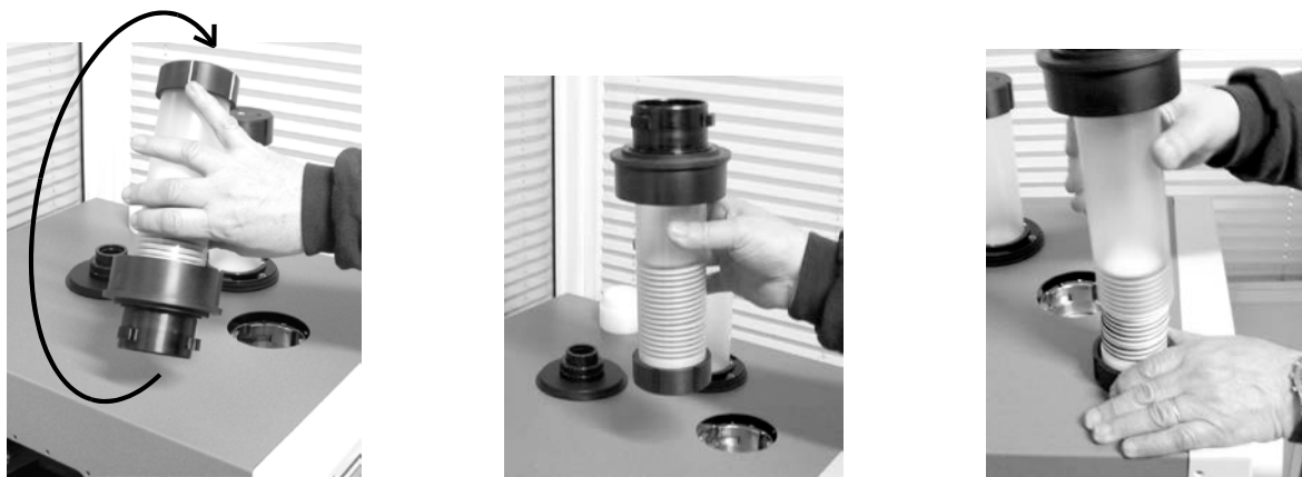
Figure 4-12. Removing Used Filters
