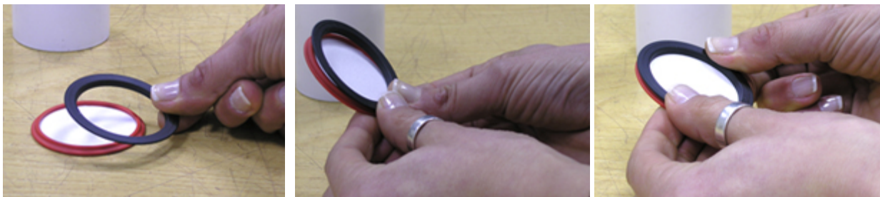
Figure 4-6. Assembling the Disks of the Filter Cartridge
