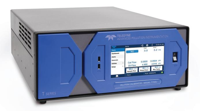
The Model T700U is ideal for the calibration of standard and trace-level gas analyzers. The T700U includes two operating modes: a high range with similar performance to the Model T700 instrument with ozone generator, and a low range which includes a "fractional mode" for producing accurate and stable  $O_3$  and  $NO_2$  levels down to 3 ppb.
