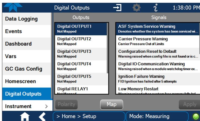
Figure 2-35. Digital Outputs Setup
