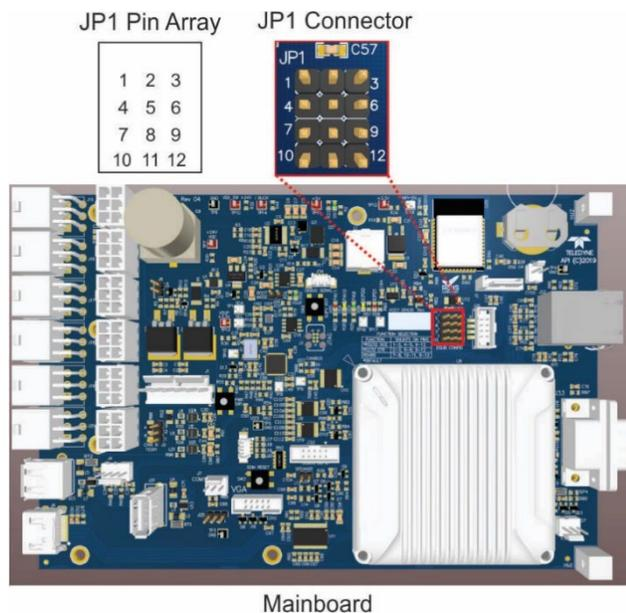
**Figure 2-6. Mainboard JP1 Location and Pin Arrangements**
