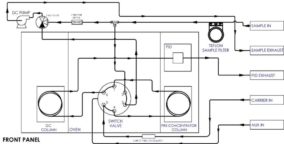
Figure 2-10. Pneumatic Flow for Sample and Injection Cycles with Standard Configuration
