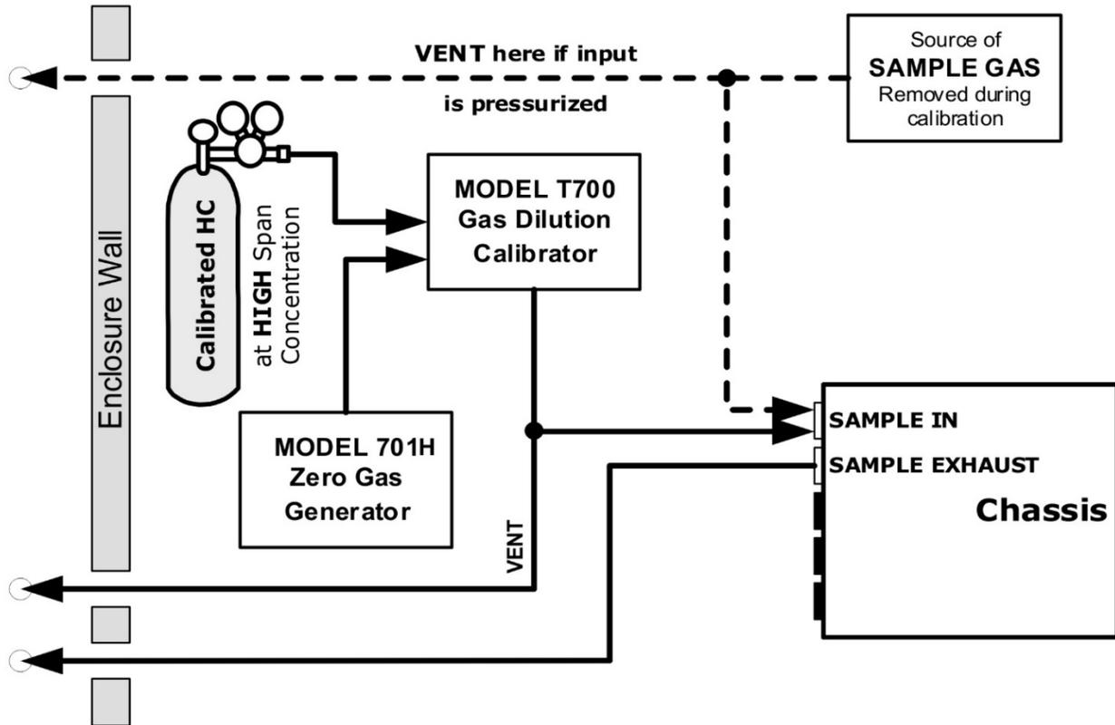
Figure 2-7. Gas Line Connections from Calibrator – Basic Configuration
