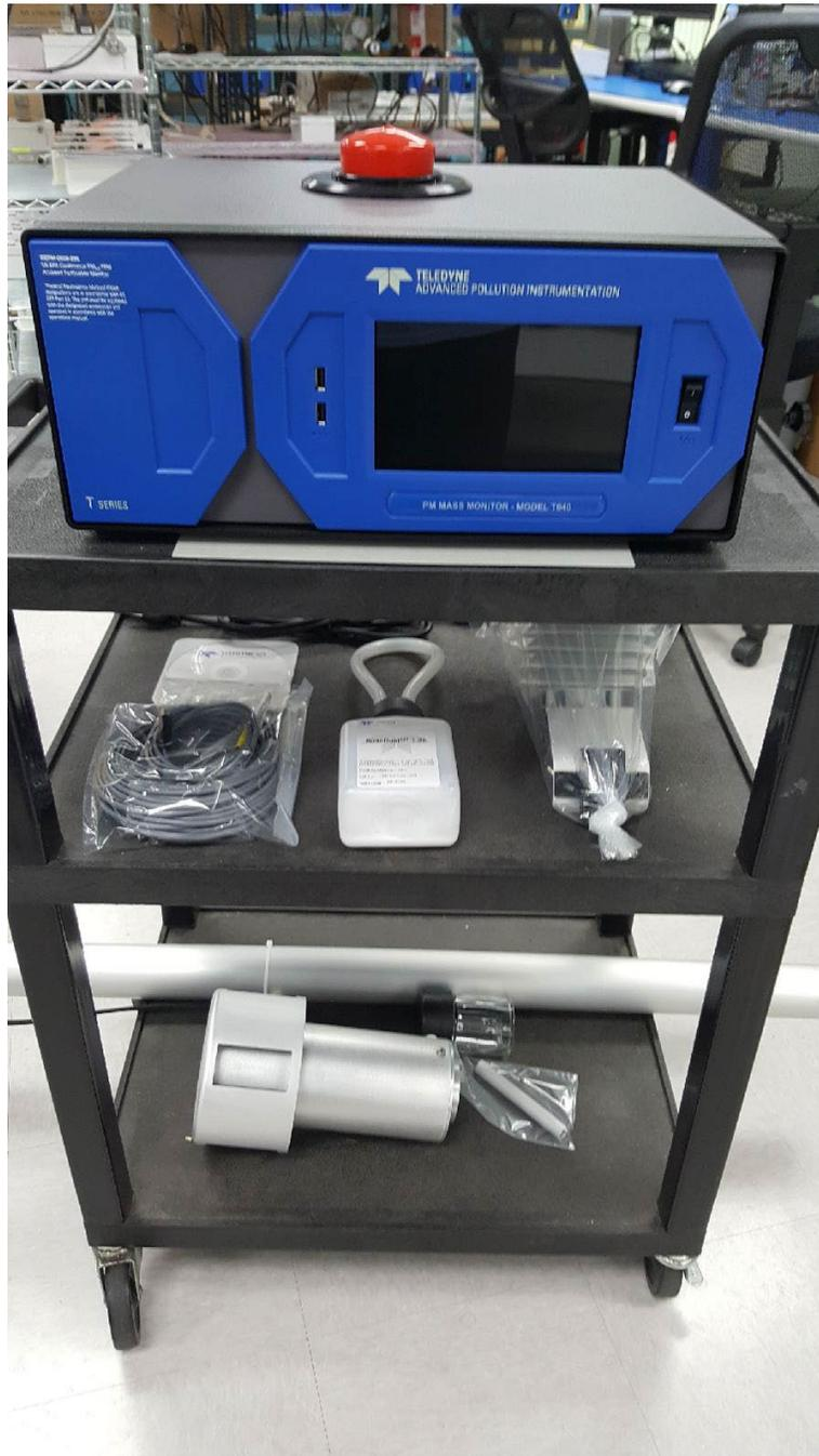
**Figure 2-1. T640 Typical Set of Included Hardware**
