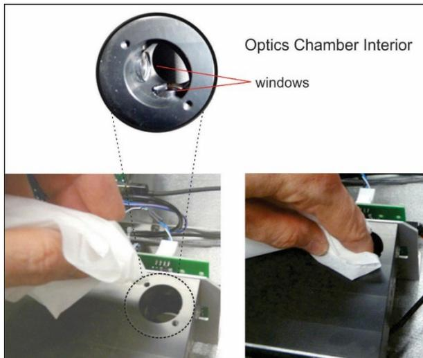
**Figure 5-6. Maintenance: Optics Chamber Windows**
