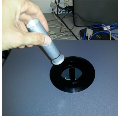
**Figure 2-8. Inlet Nozzle Adapter for ASC Connection**
