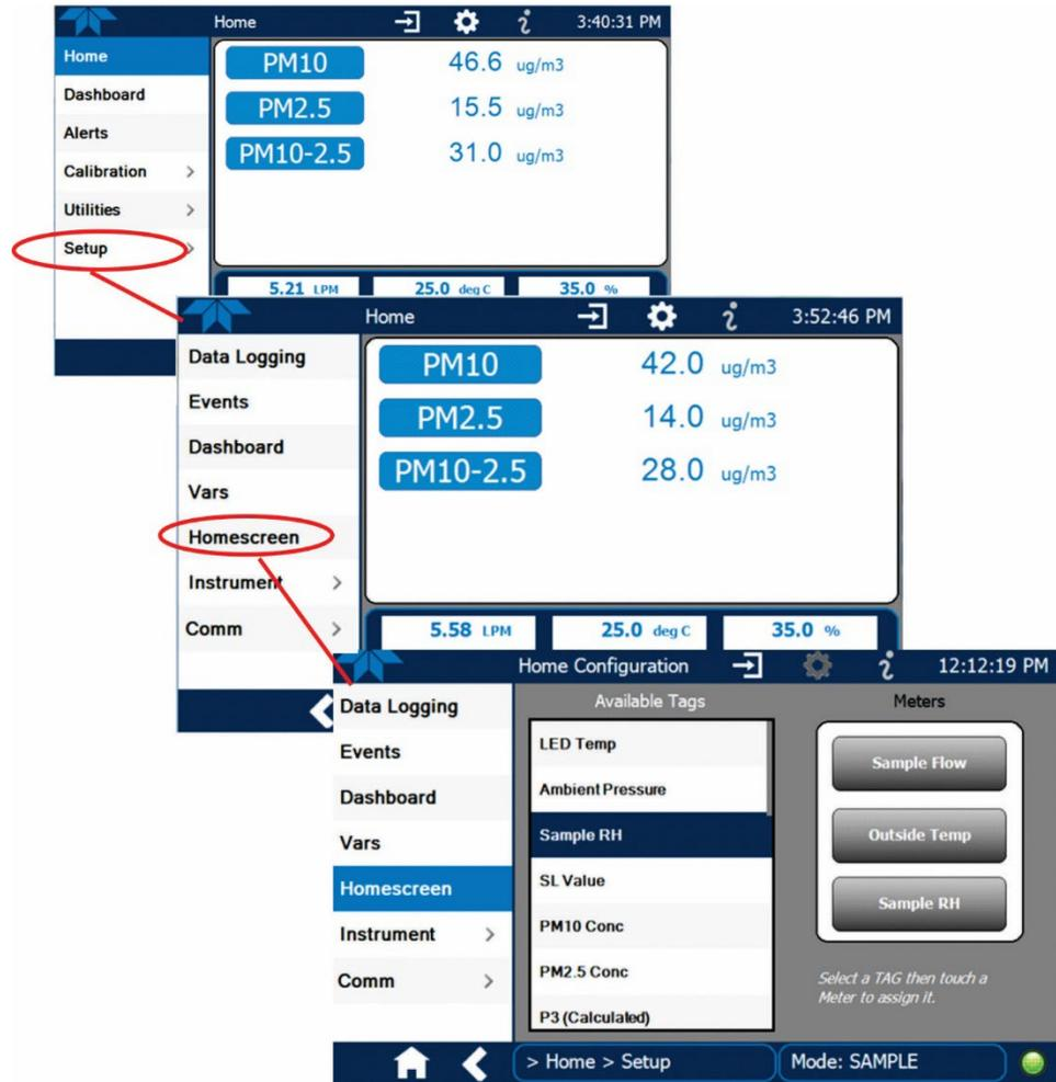
**Figure 3-21. Home Configuration thru Setup Menu**
