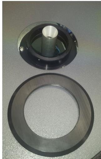
**Figure 2-9. Collar for Lower Flange**
